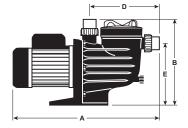
$^{\star}\,$  Suction and delivery accept 40mm PVC pipe on the I.D. and 50mm fitting on the O.D.
